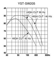
The figures below show the optimum adjustment of each control and the frequency characteristics when this subwoofer is combined with a typical main speaker system.
